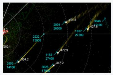
Composite digital SSR and radar tracks with weather elimination.
