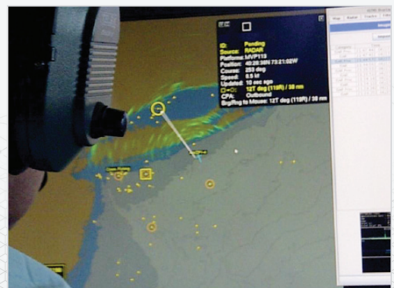
RDR-1700B(V)X SHARC display during ISAR collection.
